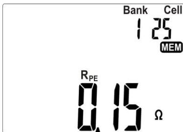
Cell is filled with the result of a single measurement.
