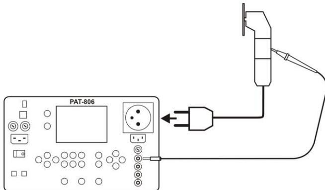
It is also possible to perform measurement without the test socket - by using the following sockets:  $R_{ISO-}$  and  $R_{ISO+}$ .
