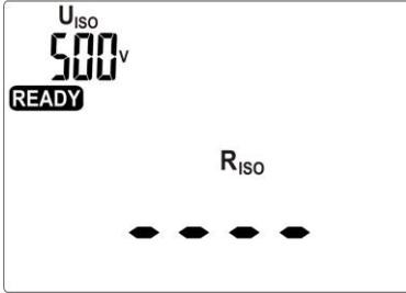
Further pressing of **R<sub>ISO</sub>** results in switching from standard **R<sub>ISO</sub>** measurement to a three-point measurement on welding equipment.
