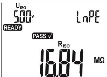
The final measurement result for all resistances above the limit values are shown below.
