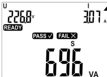
During the measurement current I is displayed alternatively with the time of measurement.
