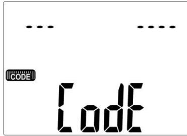
Read the bar-code of the tested device, then the meter will record the result and the code in selected memory cell, and it will proceed to the measurement screen. In order to skip reading the barcode press **ENTER**.
