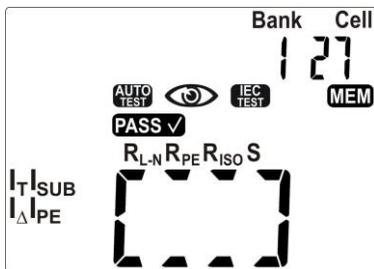
Cell is filled with the result of AUTO test.
