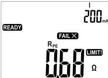
Incorrect result:  $R_{PE} > LIMIT$
