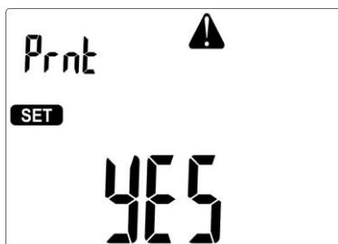
Use ▲, ▼ to set the operation of the meter with the printer (**YES**) or without it (**NO**).
