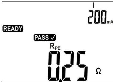
Correct result:  $R_{PE} < LIMIT$
